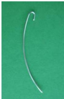
1. Use the round-nosed tool to make a 'U' shape hook at one end of the 0.6 mm wire.
