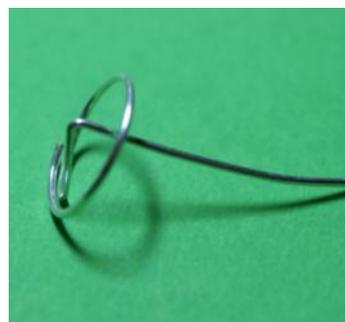
7. Bend the wire 90° again. This time so the long wire points up from the ring. Push the centre piece down gently to form the shape as illustrated.
